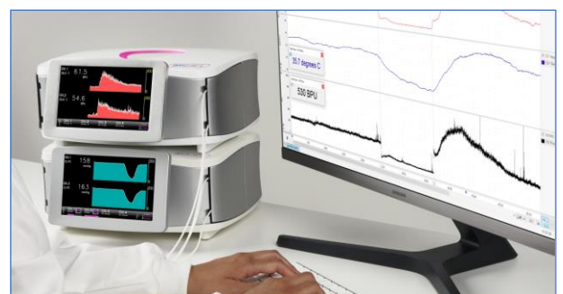
OxyLite Pro and OxyFlo Pro monitor stack for combined tissue oxygen and blood perfusion monitoring
